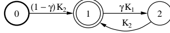
Fig. 4. Haussler's convolution kernels K_H for strings: specific instances of rational kernels. K_1 , ( K_2 ), corresponds to a specific weighted transducer over the probability semiring and modeling substitutions (resp. insertions).
