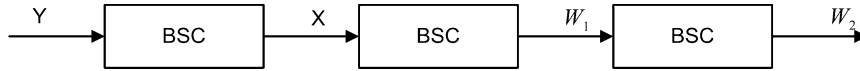
Fig. 4. The forward test channel in Region I-D. The crossover probability for the BSC between X and W_1 is D_1 , while the crossover probability \eta for the BSC between W_1 and W_2 is such that D_1 * \eta = D_2 .
